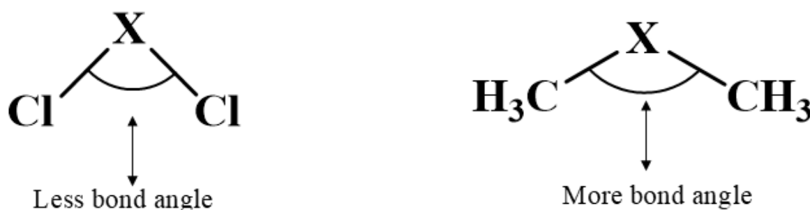
Figure: 10.1 Bent Rule Bond Angle
