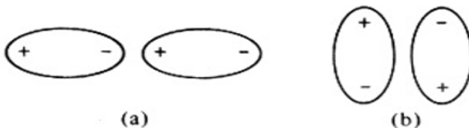
Fig. 4.1 (a) Head-to-Tail and (b) Anti Parallel Arrangement of Dipoles
